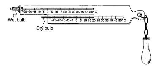
Remember: When the above sling psychrometer is swung, the water on the wet-bulb wick evaporates. This process removes heat causing the wet-bulb thermometer to drop in temperature.
